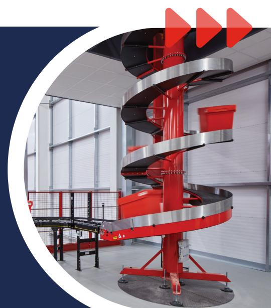
Products can be continuously raised or lowered vertically from varying levels and in areas with restricted floor space. Only one drive is required to power spirals up to 12m high. Fully reversible and twin lane options available. Spirals are suitable for many products such as cartons, containers, trays, film wrapped packs, bags, crates, totes etc.
