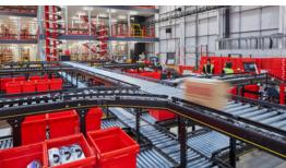
A web based WCS/SCADA was implemented by CSL to interface to the WMS system, enabling the conveyor system routing to be controlled and amended in live time. The WCS provided all historical data as well as over-arching control of the entire conveyor solution. The client has the ability to dial into the WCS from a PC/Tablet anywhere that has an internet connection.
